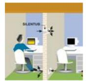
SILENTUB-100 can be flush mounted into the wall, ideal for ventilating small areas or to exchange heat between adjoining rooms.
