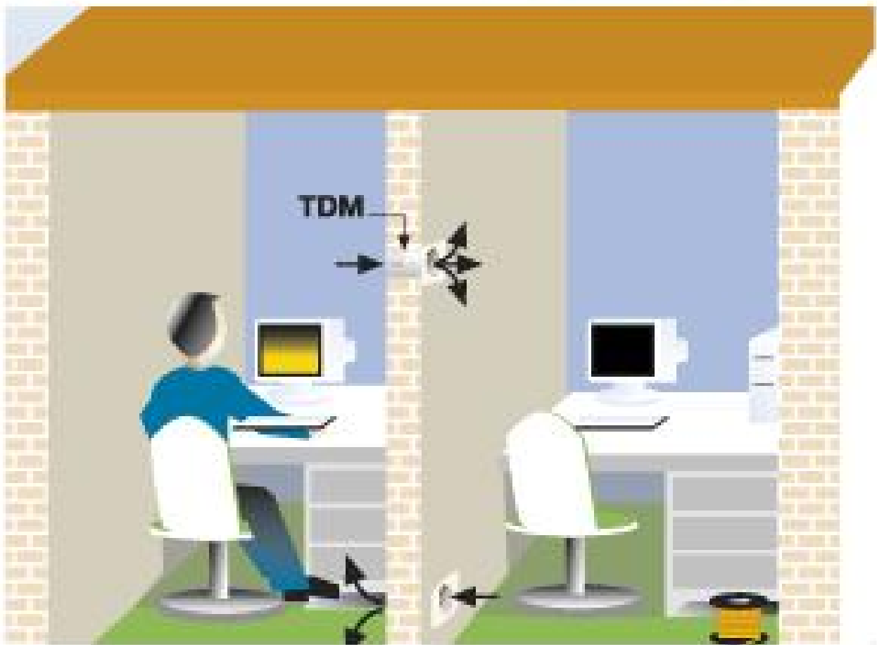
Models 100 and 200 can be installed within a wall to provide exhaust air operation or to exchange heat between adjacent rooms.
