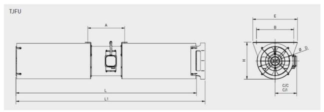
L: standard with guards, no deflector. L1: for unidirection with 1 deflector. C/C: version with terminal box (standard). C/I: version with isolator (optional).
