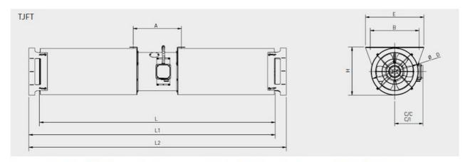
L: standard with guards, no deflector. L1: for unidirection with 1 delector. L2: for reversible with 2 deflectors. C/C: version with terminal box (standard). C/I: version with isolator (optional).
