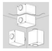
Installation at any position To be mounted in vertical, horizontal or inverted position.
