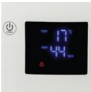
LCD screen with relative humidity and ambient temperature indicator.
