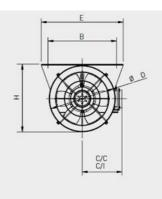
L: standard with guards, no deflector. L1: for unidirection with 1 delector. L2: for reversible with 2 deflectors. C/C: version with terminal box (standard). C/I: version with isolator (optional).
