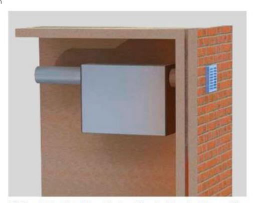
PIV W unit takes the air from the façade [preferably oriented to south], passes air via a anti-insect filter and supplies it into the dwelling via hallway.
