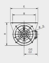
L: standard with guards, no deflector. L1: for unidirection with 1 deflector. C/C: version with terminal box (standard). C/I: version with isolator (optional).
