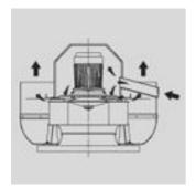
**Self cooling system**Special design in order to cool the motor and to extend the life of the assembly.
