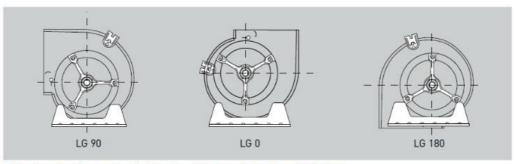
Mounting feet (accessory) allow 3 positions of the inlet discharge.
