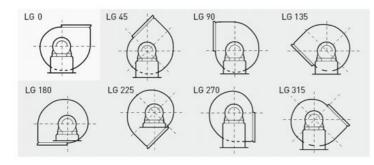
LG 0 standard supplied position. Other LG positions and RD configuration manufactured on request.
