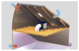
PIV unit takes the air from the attic, where temperature is always higher than external air, passes air via a filter and supplies it into the dwelling via hallway below attic. It has available a pre-heating battery for the new air, for cold seasons. If the attic temperature is higher than 25°C, the ventilation stops.
