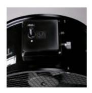
Flame retardant terminal box Wiring terminal box inflame retardant plastic V0 fixed to the exterior of the casing and provided with a two-pole On/ Off switch</strong>. Cable gland PG-11
