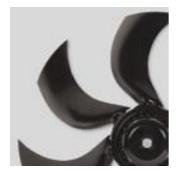
High efficiency "Sickle blade" impeller Designed to ensure the highest and most efficient airflow performance with the lowest noise level. Dynamically balanced to ISO 1940 standard. Manufactured from aluminium plate;  $\emptyset$  250 to 355 models which are manufactured from pressed sheet steel.
