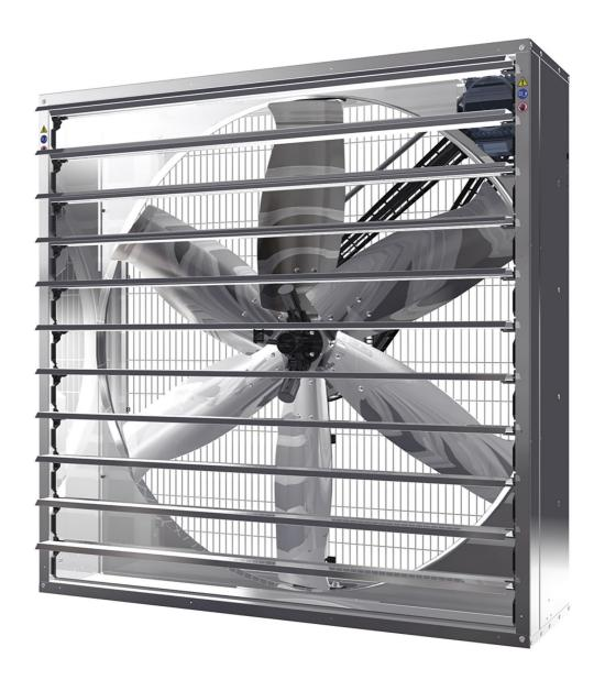
Outlet louvre shutter with automatic opening when switching on the fan, to avoid its opening when it is not working.
