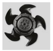
**High efficiency "Sickle blade" impeller** "Sickle Blade" impeller specifically designed to ensure the highest and most efficient airflow performance with the lowest noise level. Dynamically balanced to ISO 1940 standard. Manufactured from pressed sheet steel.
